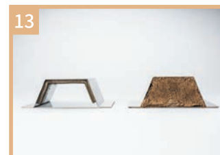
13 発泡充填材 閉断面を充填し、車室内静粛性を向上させる発泡充填材 Pumpable Sound Insulator Expands and fills in closed section for a silent cabin.
